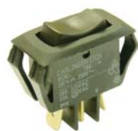
SPDT on-off-on rocker switch 16A 125VAC 10A 250VAC, 3 terminals approx. base size : 1/2 x 15/16"
