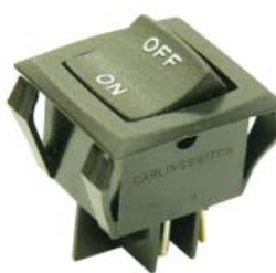
DPST on-off rocker switch 16A 125/250 VAC / 10A 28VDC 4 terminals, ref. # 260011E approximate base size : 7/8 x 7/8"
