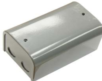
relay enclosure heavy gauge sheet metal four 1/2" knockouts size : 5-5/16 x 3-3/8 x 3-1/8" high
