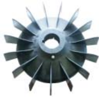
Fig. C plastic, tightens with metal ring on tapered hub
