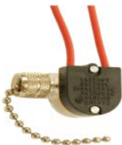
pull chain switch, 1 speed on-off SPST, 6A/125VAC
