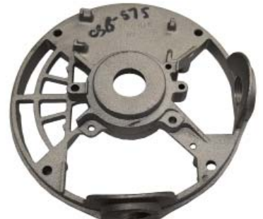
non-drive end bell, open, brg size 6203 threaded conduit hole
